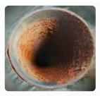
The cooling water inside closed systems is not dynamically evaporated. It only serves to transfer heat. Softened water is generally used for this purpose. It does not produce any limescale or mineral deposits, but it is very **corrosive**. Conditioning agents for closed cooling circuits consequently put special demands on **corrosion inhibitors** for protection against corrosion.
